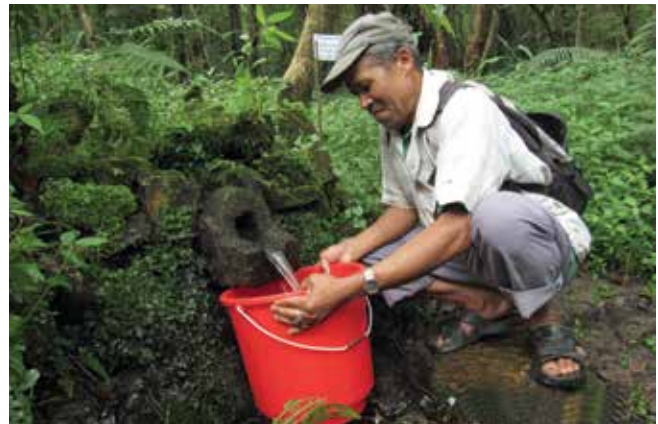
Figure 25: Discharge measurement using bucket and stopwatch method
